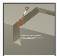
Do foundation benches below the depth of ground Frost.
