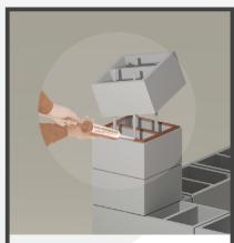
Place all elements of the fence using suitable mounting glue, so that all welds are sealed.
