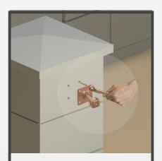
Drill the holes in the post and then fix the hinges using a chemical anchor. Fix the spans and gates on the hinges.
